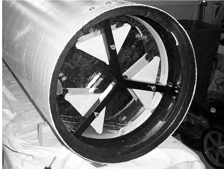
Figure 1. Mirror cell of a 17.5-inch mirror.
