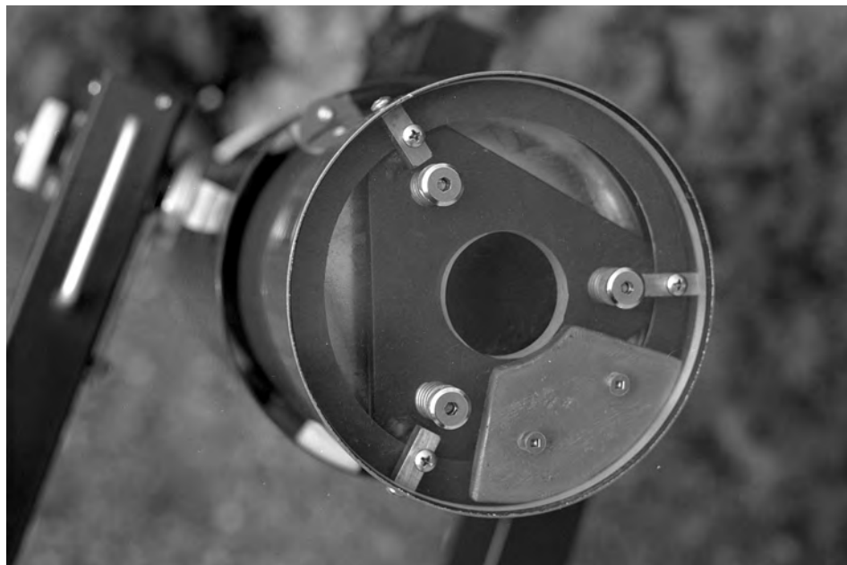
Figure 1 — Rear view of the mirror mounting support structure.
