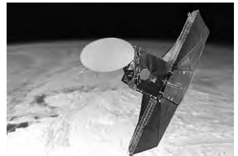
The ODIN spacecraft has been placed in a Sun-synchronous orbit some 600 km above the Earth's surface. In this fashion it will track along the Earth's day-night terminator with its solar panels constantly directed towards the Sun. Further images and spacecraft details are available at www.iras.ucalgary.ca .
