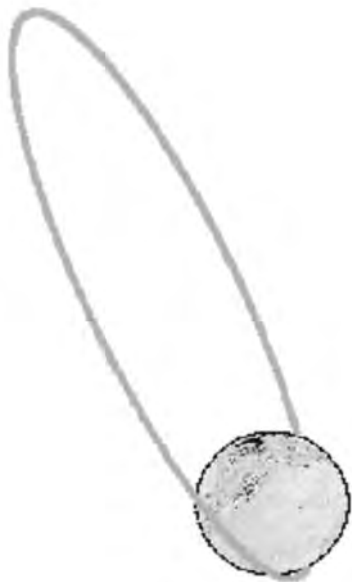
The orbit of a typical Molniya satellite. The high altitude at apogee ensures a long observing opportunity for satellite trackers in the Northern Hemisphere.
