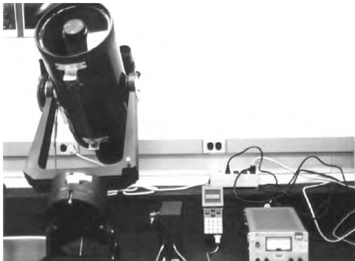
The Meade 10-inch Schmidt-Cassegrain reflecting telescope is seen with the equipment used to control it. This was the primary satellite tracking system used by SSRAL until its more advanced system went online on January 29, 2000.
