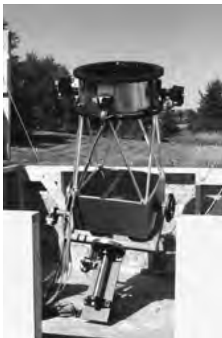
The telescope at The Iwanika Observatory, which is presently a 10-inch f/4.5, will eventually operate as a semi-robotic 18-inch f/5.
