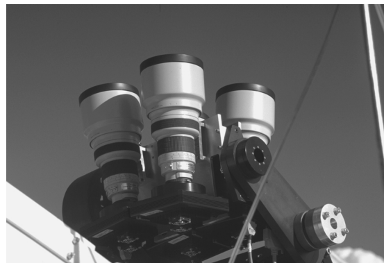
The Robot Optical Transient Experiment (ROTSE) on the roof of a modified military communications enclosure at Los Alamos National Laboratory in New Mexico. The enclosure was previously used in the Gulf War, and obtained by the researchers from a scrap-metal dealer for $250. The entire enclosure, which houses the computer that drives ROTSE, can be picked up with a forklift truck and moved to any location accessible by road.
