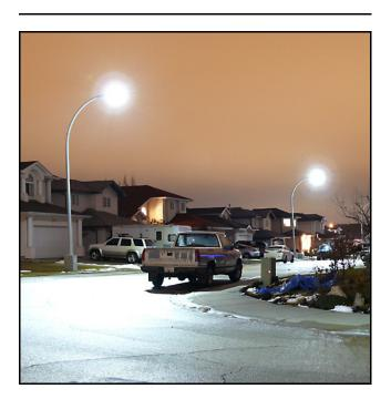
Pedestrians can see more clearly and feel safer with the reduced glare and near-white light produced by LED lights in a full cut-off luminaire.
