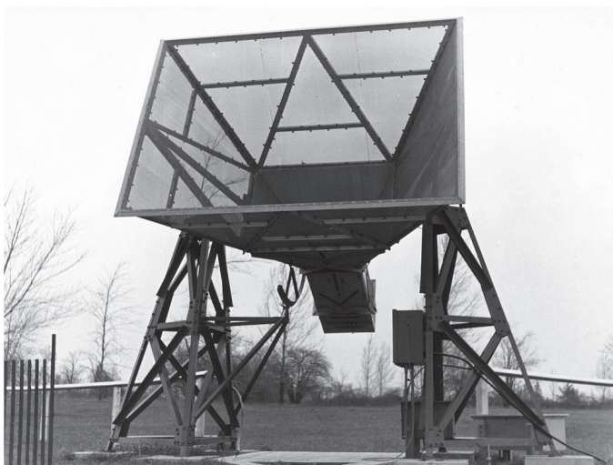
Figure 7 — A close up of the west element of the pyramidal horn antenna interferometer used for the Cas A absolute flux measurements and the antenna used for measurements of the absolute brightness of the North Celestial Pole at 320 MHz. The dimensions of the aperture are 2.76m x 3.70m. This type of antenna was used because its electrical collecting aperture area can be readily computed from the electromagnetic theory of waveguide apertures (reproduced courtesy of the Department of Astronomy & Astrophysics, University of Toronto).
